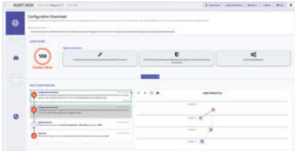
Claroty CTD alert view showing root-cause analysis and chain of events
