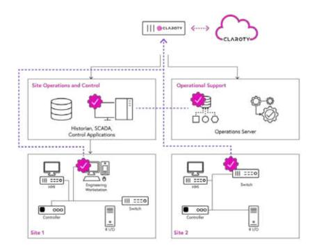
Claroty Edge deploys as a lightweight executable on Windows and Linux hosts to automatically query assets on the local subnet. In air-gapped environments, Edge can deploy to Linux-based devices via Docker containers, eliminating the need for host devices.
